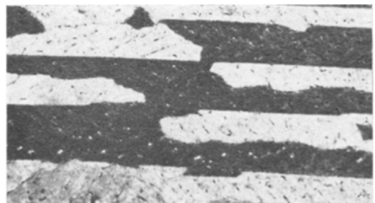
Figure 9 Micrograph showing how the twins change sides ( \times 400 ).
